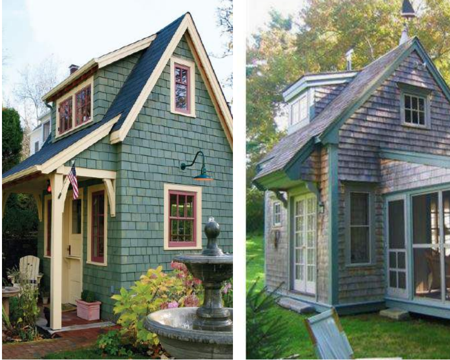
Figures 10 and 11: Use of trim around windows and accents on corners and edges
